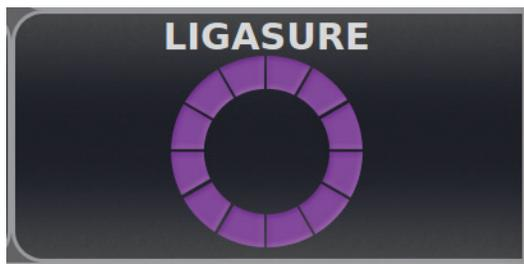
During instrument activation, the progress wheel in the LigaSure display control panel illuminates, and a tone sounds for the duration of energy delivery.
