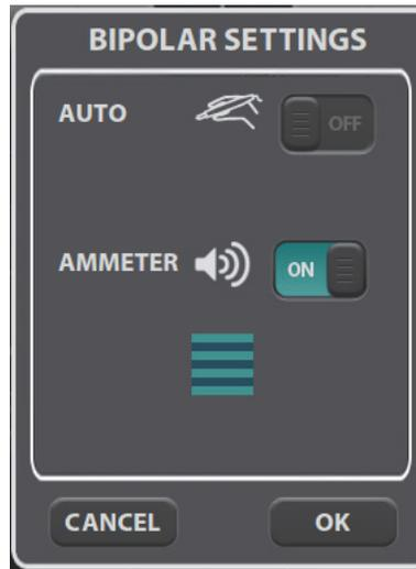
3. Touch **OK** to close the ammeter settings window and retain any changes. The visual ammeter is added to the Bipolar screen and the audio and visual feedback is in use during Bipolar activation.
