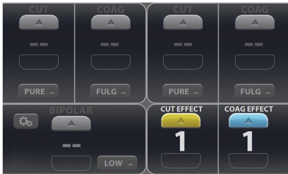
The Bipolar Resection screen has controls for both CUT and COAG modes. The effect setting may be adjusted for either mode from 1 to 6—1 being the minimum effect for the selected mode. During instrument activation, the Bipolar Resection screen illuminates brightly as yellow for CUT and blue for COAG. A tone sounds for the duration of energy delivery.
