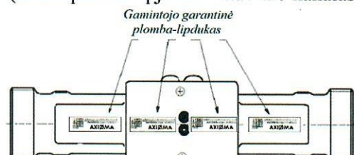
d) srauto jutiklio q_p = 10/15/25/40/60 \text{ m}^3/\text{h} plombavimas
