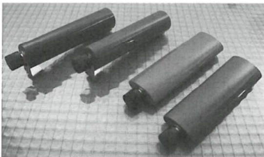
Fig. 2: PCDs, round and oval construction
