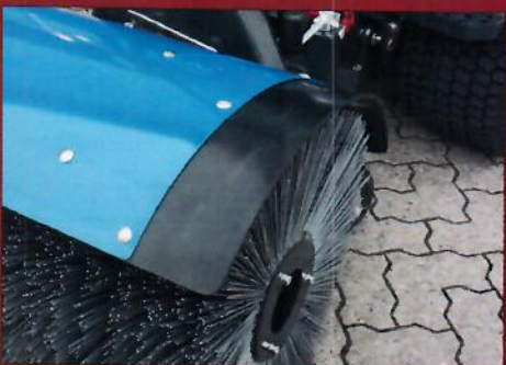
The brush guard is equipped with rubber edges that protect against damage in the event of a collision.
