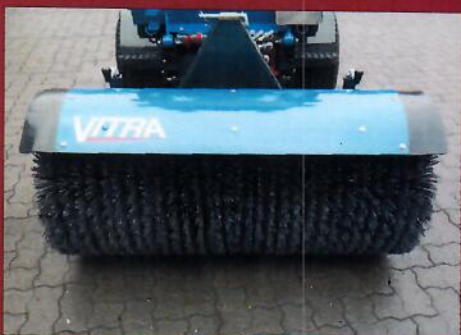
Splitting the two brush roll halves saves a lot of time and ensures a quick replacement of brush rings.
