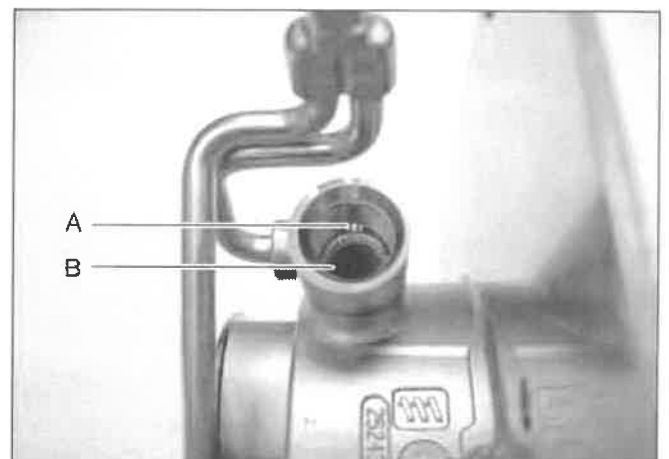
A Ignition air drillhole B Glow pin socket with lining installed
