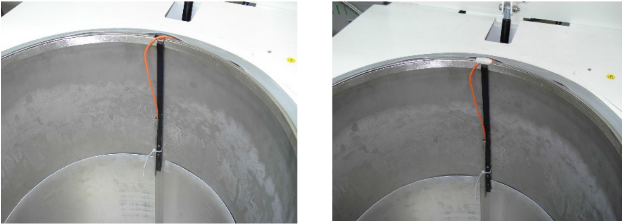
Figure 22. Pt100 (-200 °C to + 50 °C) for nitrogen/cryogenic tank
