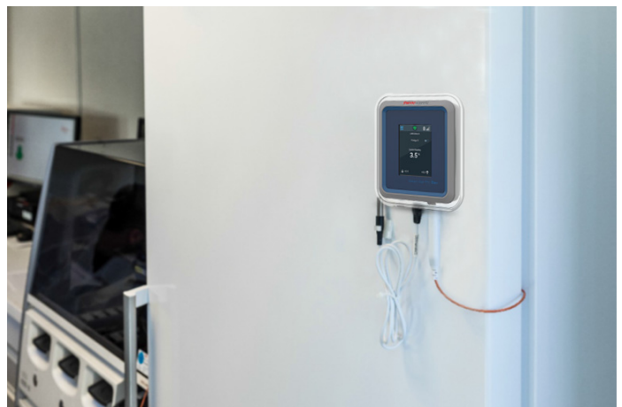
Figure 26. Smart-Vue Pro Duo/Quatro data logger mounted on the refrigerator door
