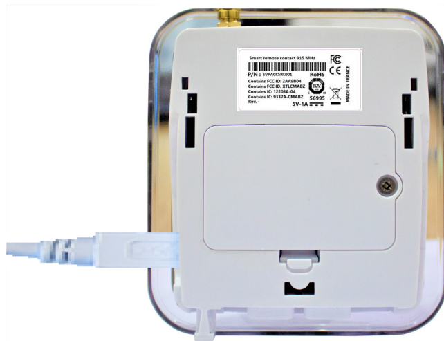
Figure 74. Optional: plug data logger into AC (USB) power to avoid losing data
