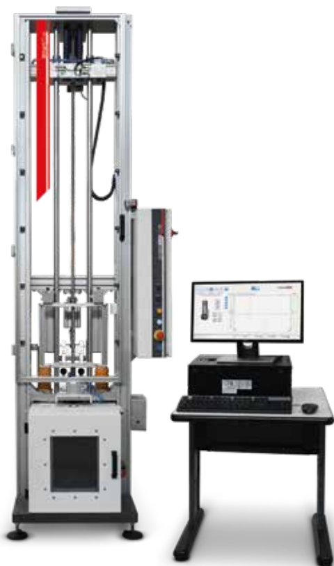
Drop Weight Tower DW1000 with climatic chamber
