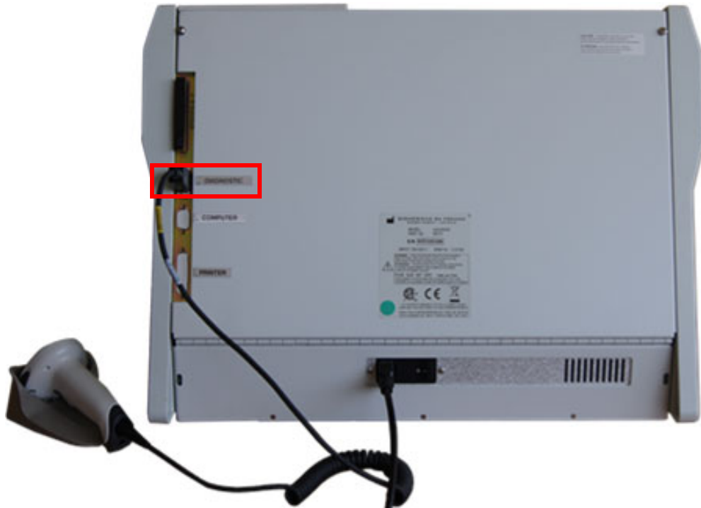
Figure C-2: Location of diagnostic port
