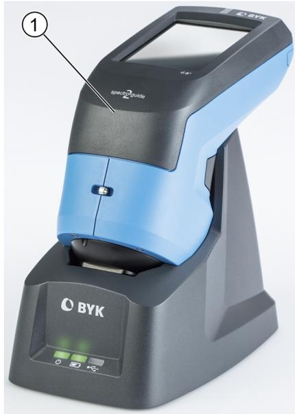
1 Instrument inserted in docking station
