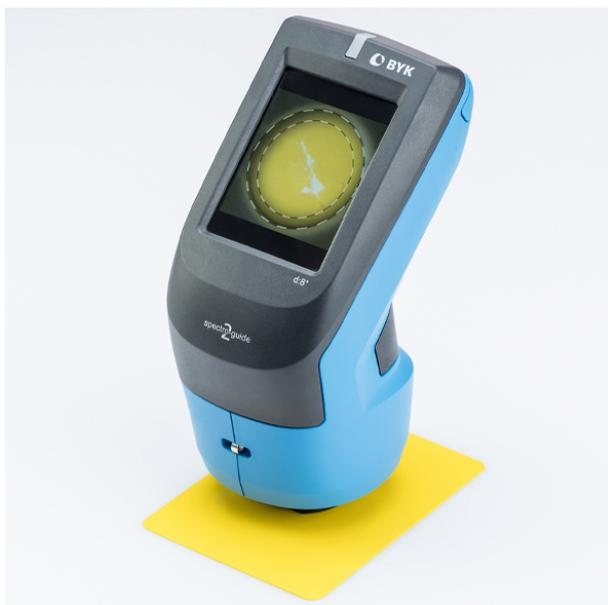
By placing the base plate of the unit onto a surface and pressing either the **Operate** button on the rear side of the instrument or triggering the measurement on the display, the instrument measures the surface and processes, displays, and stores the measured values.
