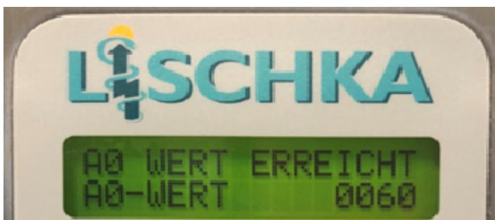
Once the recooling is done and program finished, a message will display that the A0 value set (in this case (A0-60) was reached. This message will stay displayed until someone opens the door to remove the goods.
