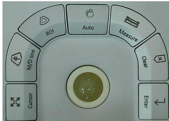
1. Measure: activates measurement caliper and current measurement and calculation setting.
