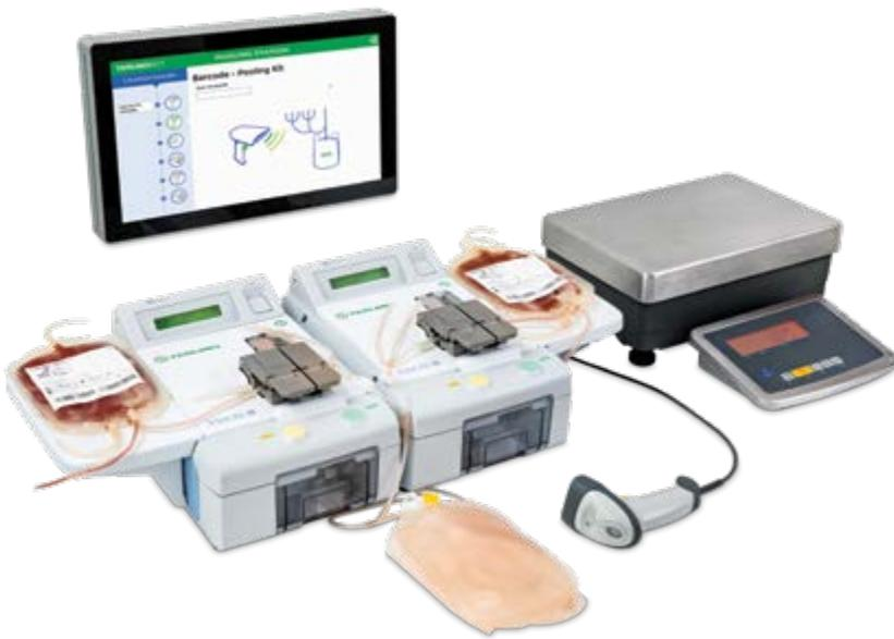
The TSCD-II is a closed-system welder suitable for a wide range of lab applications. Designed for quality and flexibility, TSCD-II creates reliable, strong, consistent welds using PVC tubing in various combinations of wet and dry. TSCD-II can be used across your blood center to perform tasks including:
