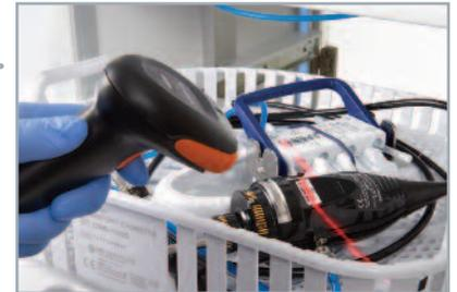
Barcode scanner for ease of endoscope and operator identification
