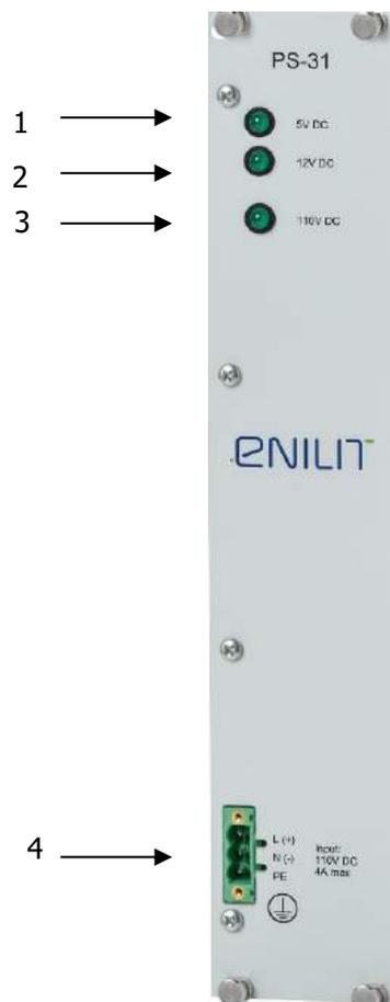
Figure 9. Power supply module, Front view
