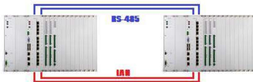
Figure 231. Example of connections between redundant RTUs
