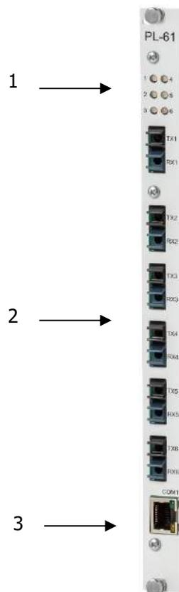
Figure 20. Figure 3.19 Plastic fibre optic module, Front view
