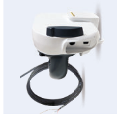
Amika Holder Com Nurse Call (Delivered with Amika Nurse Call Cable) To connect Amika/ Applix to a Nurse call system. Pump alarms states are automatically reported.
