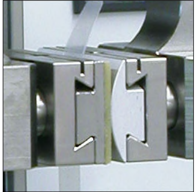
Jaws, convex aluminum against smooth vulkollan
