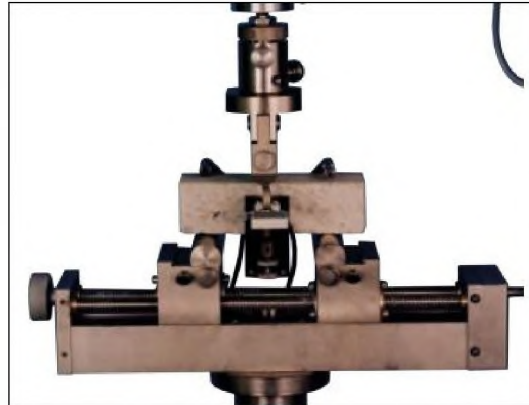
Picture 19: The Type B flexure table (Item No. 317121) can be adjusted via the lead screw. Top connection here is via an adapter, bottom via a connector.
