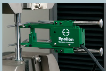
Model 3542 with round metal specimen
