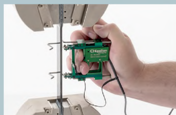
Model 3542 Quick Attach feature enables mounting with one hand
