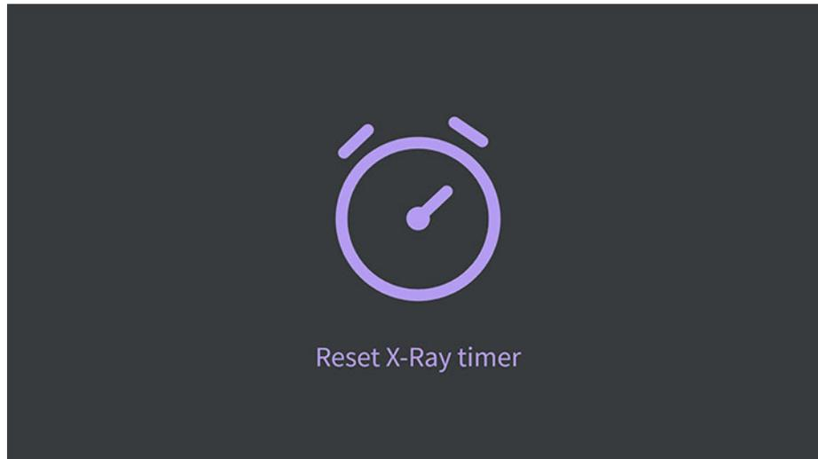
The **X-Ray Time Reset** screen is displayed on the Touch Panel ([10.3.6 X-Ray Timer on page 240](#)) and blinks. Press anywhere on the screen to reset the X-Ray timer after the elapsed duration.
