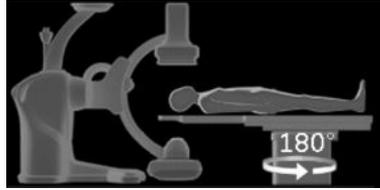
The patient position relative to the table top does not change when the table is rotated so there is no need to reselect a patient position on the DL screen.
