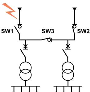
Source changeover between 2 incoming lines (SW1 and SW2) and a busbar coupling switch (SW3)
