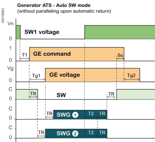
Case ①: Generator channel closing after Generator power on (configurable option)
