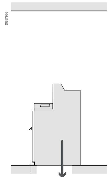
N.B.: parts for guiding the gases to vent openings and cooling walls are not part of the switchgear supply. These must be adapted to each specific case.
