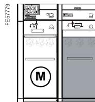
(M): The circuit breaker function is motorized
