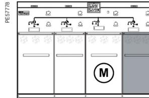
(M): The circuit breaker function is motorized
